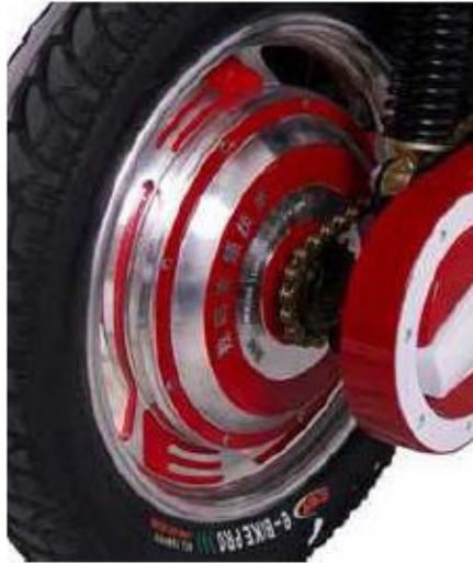
BLDC Hub Motor used in e-bike application
